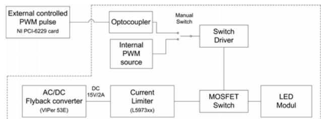
Figure 3. Block diagram of manual / automatic LED intensity regulation for 3W module
