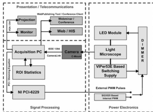
Figure 1. A design of high speed imaging workstation with light microscope
