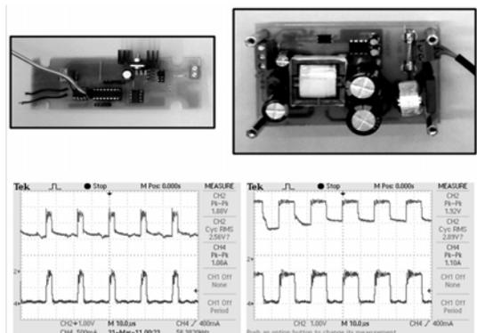
Figure 5. Dimming board, Flyback supply and two impulse drain currents, measured power illumination characteristics
